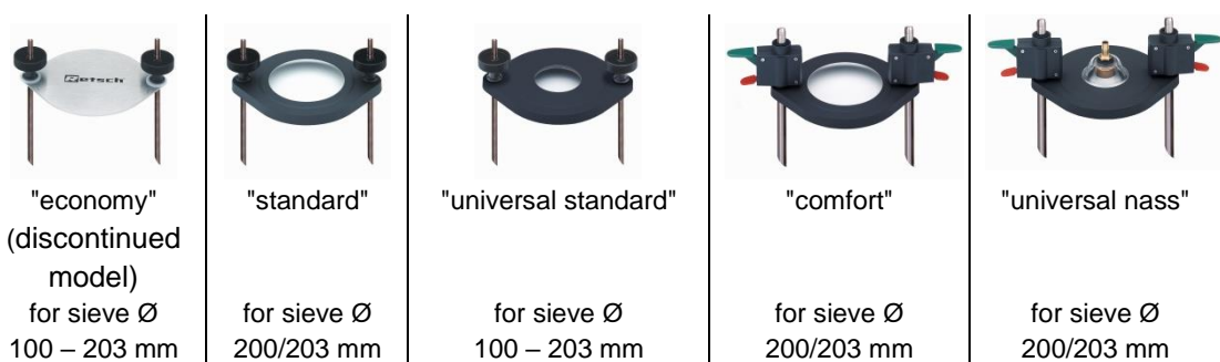
Fig. 3: Types of the sieve clamping unit
